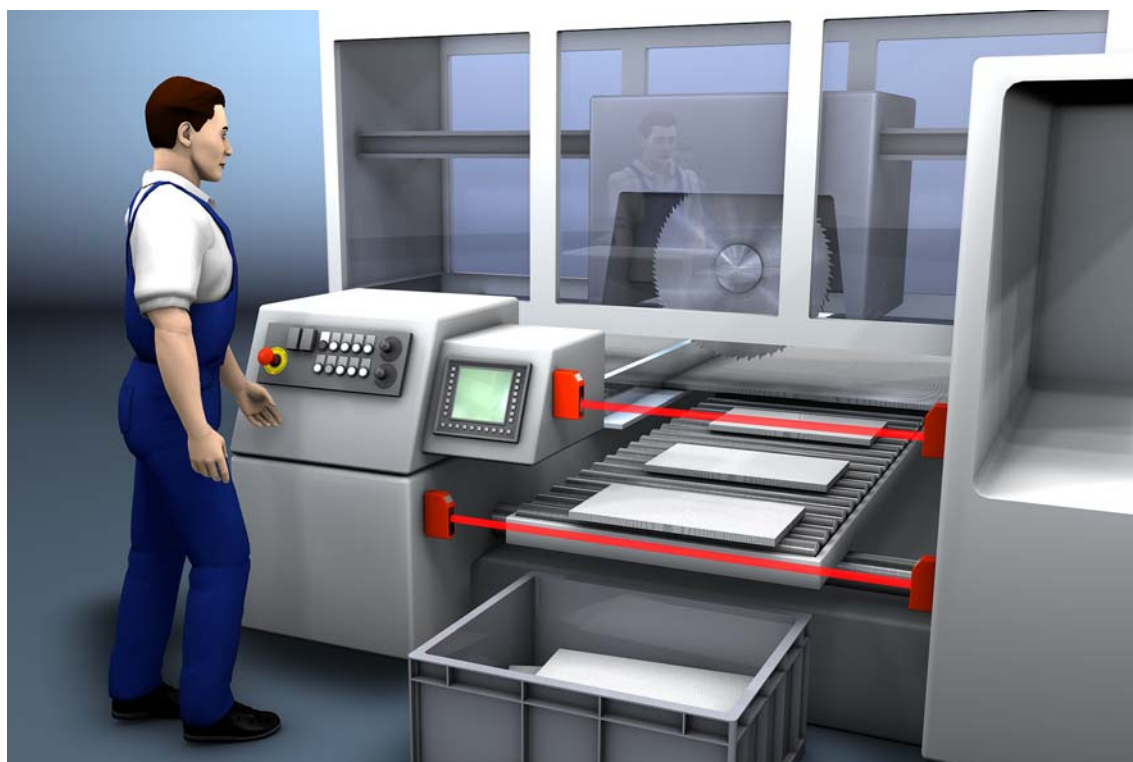
Figure 5.2: Access guarding / intervention control on sawing machines
