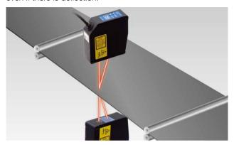
**Substrate tilting/warpage measurement** Diffuse-reflective type By calculating measurement results from two sensors, substrate tilting measurements can be performed. The two sensor units can also perform measurements separately.
