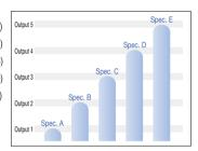
By performing settings such as these, output 1 will turn on for workpieces of Spec. A and output 2 will turn on for workpieces of Spec. B, while no output will turn on in the case of workpieces that do not fit the set Spec. (such as defective items). Settings such as these are not possible using the HH/HI/LO/LL setting method.
