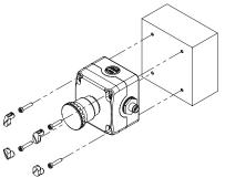
The wall fixing screws and the ones for closing the housing cover can be sealed with 4 caps (supplied with the housing). The caps not only give the housing a more pleasant look, but they also prevent the accumulation of dirt inside the recesses of the screws besides making tampering more difficult.
