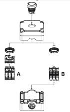
The housing can fit up to 3 contact blocks/LED units (E2 CP, E2 LP) for panel mounting by means of a mounting adapter (A) or up to 3 contact blocks/LED units (E2 CF, E2 LF) for base mounting directly on the bottom of the housing (B).
